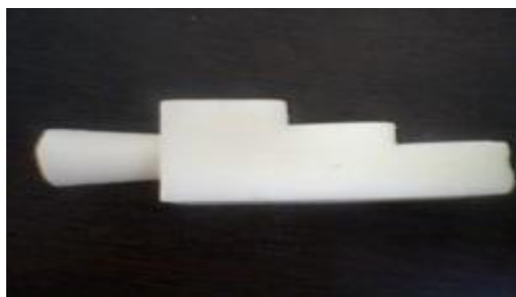
Fig 2 Typical wax pattern
